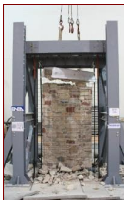
Strengthened using injection 0.60g
