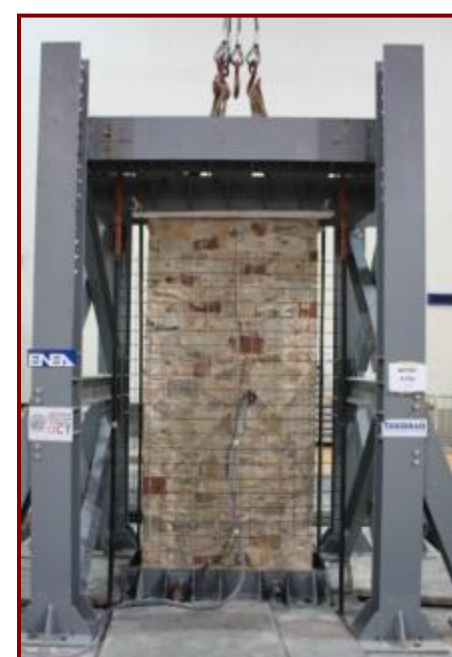
Strengthened using ties and injection 0.75g
